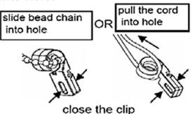
2. Leave tensioner locking on the chain/cord before installation.
