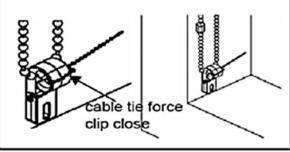
4. Fasten screws, then cut off the cable tie and dispose it properly.
