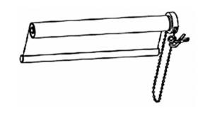
3. Before install tensioner on mounting surface, use cable tie to close the clip. Locate tensioner properly, holding the chain/cord loop taut but allowing chain stopper go through.
